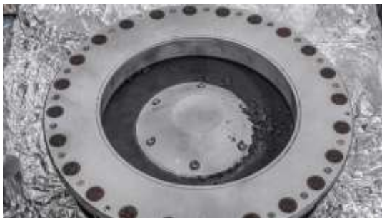
Returned capsule after heat shield opening with debris from asteroid Bennu on the outside of the OSIRIS-REx sample collector head Screenshot: NASA TV and [1]
